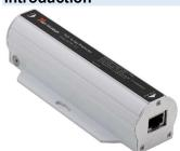
SP PR10G is a single port PoE surge protector, with 1 input port and 1 output port, support 8 lines network signals and PoE Surge protection. It is designed to handle differential mode surge voltage (8/20us) 4KV and Common mode surge voltage (8/20us) 6KV, and support 100/1000Mbps.
