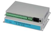
The RS485 Hub transforms RS485 bus into star topology making RS485 a dependable network. Each RS485 Hub Port is Isolated from the other and support 1.2Km run of multidropped RS485 devices. Additionally, the Hub ports are Optically Isolated, Short Circuit, Surge & ESD protected rendering ruggedness to your network. In case if any there is a cable fault or a RS485 device failure or a shorting in the network, the problem is restricted to only that ports of the Hub. Connect with ease as many as 256
